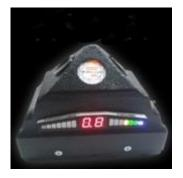
Function: The device will detect an object up to 4 feet away using an lcd display on the front and it will indicate if the object is on the left or the right of the unit
