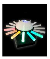
Function: This device is basically a triboelectric energy detector which is the principal of static electricity. This meter visually follows triboelectric fields horizontally. The triboelectric effect is not very predictable and therefore this device is not a consistent detector as say an emf detector might be.
