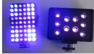
**Function:** UV/IR lights are used in conjunction with our full spectrum camcorder to be able to film in the full spectrum of light.
