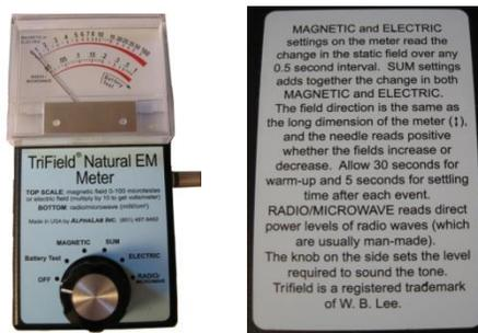
**Components:** The tri-field meter has a knob that turns the meter on and is a selection switch for the function you wish to run the meter. The choices are a test of the battery, magnetic mode, sum mode (combination of magnetic & electric modes), electric mode and radio/microwave testing. The silver knob on the side selects the units' sensitivity. The unit measures in hz, mG & volts/meter. See the units spec sheet for additional information.
