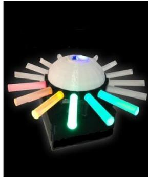
**Function:** This device is basically a triboelectric energy detector which is the principal of static electricity. This meter visually follows triboelectric fields horizontally. The triboelectric effect is not very predictable and therefore this device is not a consistent detector as say an emf detector might be.
