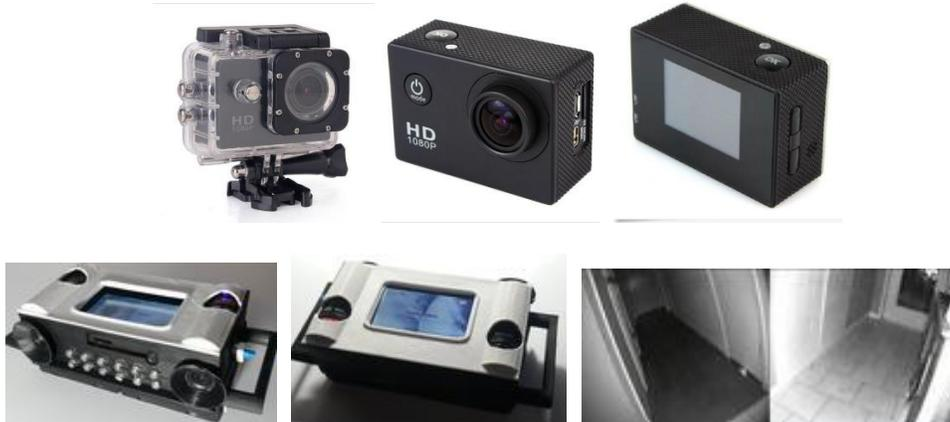
**Function:** Stand alone cameras are commonly known as ‘drop cameras’ because these cameras maybe ‘dropped’ off at any given location due to their portability. The Go Pro clones can take both still photos and video. The twin camera captures 180 degrees of footage all on one screen. The 2.7" split LCD Screen allows for viewing both camera's live. Both styles split recordings into 2 minute segments for ease of review.
