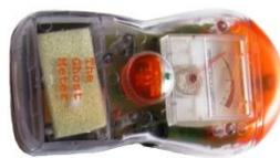
**Components:** Meter and battery compartment. Meter measures in mG in the range 0 – 5 mG
