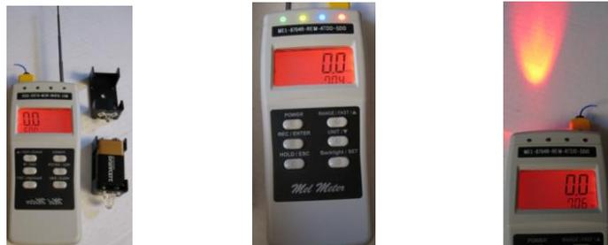
**Components:** The MEL meter has an external radiating antenna, fast response type 'K' thermal couple temperature sensor and shadow detection probes (2). Mel meter measure in 200; 2000 or 20,000 mGauss or 20; 200
