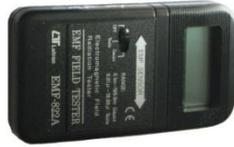
**Components:** Meter can measure in milligauss or tesla via a selection switch. Meter has a range of 0.1m~199.9m gauss or 0.01 $\mu$ ~19.99 $\mu$  Tesla.
