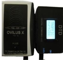
**Function:** The Ovilus X is an electronic speech-synthesis device which utters words depending on environmental readings, including electromagnetic waves.
