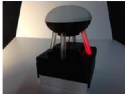
**Function:** This device is a visual ambient temperature sensor with 2 ambient probes that are constantly comparing the difference in air temperature. It picks up changes in the ambient air temperature and displays the change using a blue light for cold, and a red light for hot. The device automatically resets every 30 second's if the ambient air temperature has remained a constant temperature.
