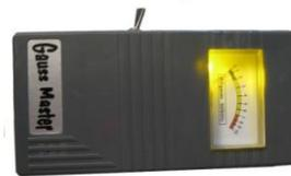
**Components:** Meter measures milligauss in the 50/60 hz range which is 0-10 milligauss. This unit was modified to add a led and a on/off switch. The original timed off which was not conducive to leaving the meter on and in a location.
