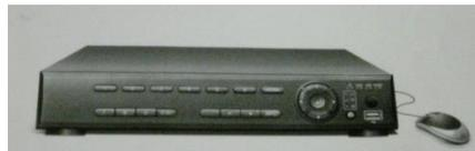
**Function:** The DVR or digital video recording system is used on investigations to monitor and record activity in various locations simultaneously. Since the cameras are night vision capable the system can monitor in total darkness. This system is used when ac current is available.
