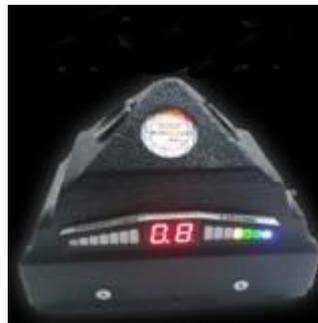
**Function:** The device will detect an object up to 4 feet away using an lcd display on the front and it will indicate if the object is on the left or the right of the unit
